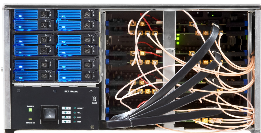
Front access to hot-swap removable SSD tray and Front access to removable process board for ease of maintenance
